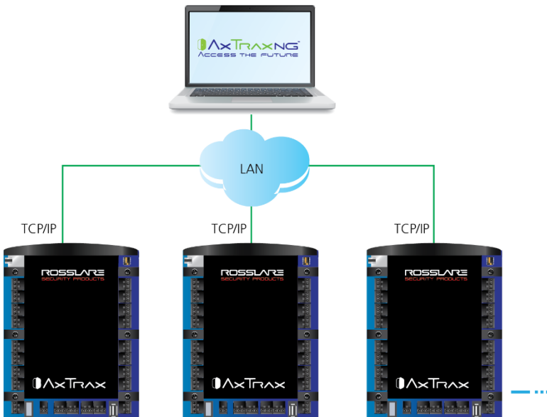
Figure 23: Connecting Multiple Access Control Panels (AC-825IP) to the AxTraxNG Server
